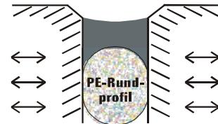
We recommend masking the edges of the joint with masking tape to ensure a clean and straight joint. The sealant must be sprayed in such a way that sufficient pressure is exerted on the joint flanks. Smooth the pressed-in sealant with a suitable joint spatula before skin formation. For smoothing joints, our smoothing compound Wikofix GM 52 has proved its worth in practice.
